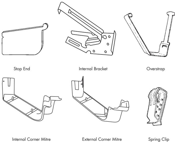
Note: Internal and external corner mitres are only available for the 115 Quad Gutter
