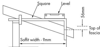
Note: The top of the fascia should be located as follows: metal roofs - 2mm (min) below the roof sheeting. Tile roofs 35 to 65mm above the top corner of the rafter.
